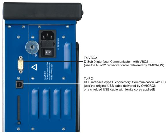
Figure 3-4: Interfaces to VBO2 and PC
